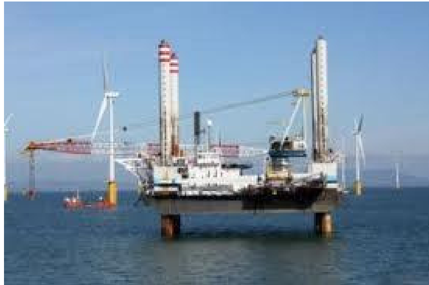
A2Sea Sea Worker[self elevating Turbine installation vessel]
